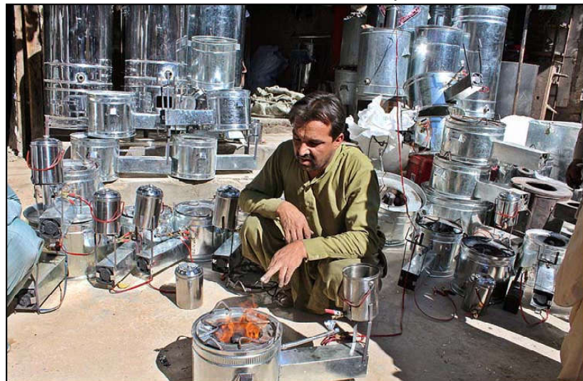
QUETTA: A vendor demonstrates igniting of locally made heater. This newly launched heater is low in cost and could be used with the used oil.
