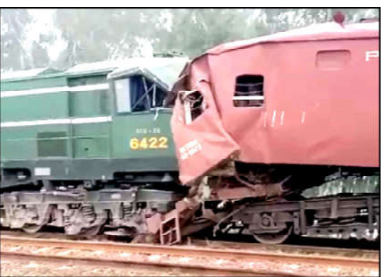
SHEIKHPURA: A view collision between Mianwali Express with goods train near Qila Sattar Shah railway station
