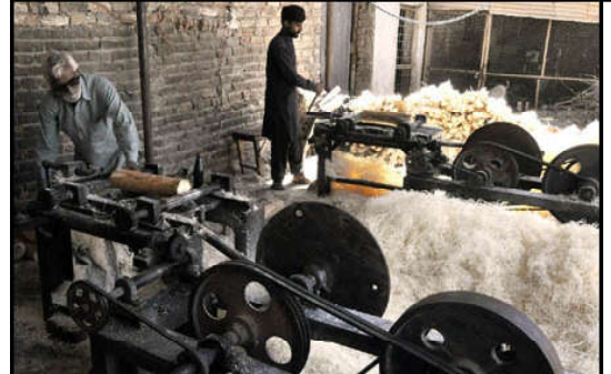
RAWALPINDI: Workers busy producing khas from wood pieces with the help of machine to be used in making of room cooler at his workplace.
